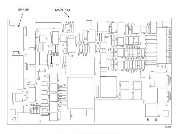
Figure 2-12. Main PCB (Model 132) EPROM Replacement
